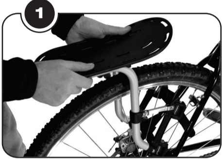
Start by placing the rack in position on the front or rear of your bike.
