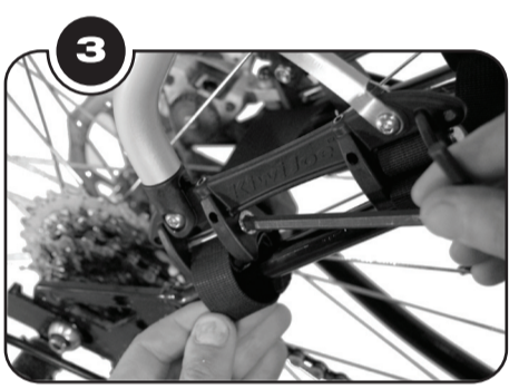
Use the ball-end of the 5mm allen-key to tighten and take up the slack in the strap.
