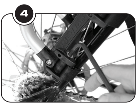
Now turn the 5mm allen-key over and use the short end to tighten securely.
